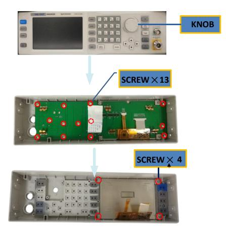
Figure 4-5 Removing the LCD and keyboard
