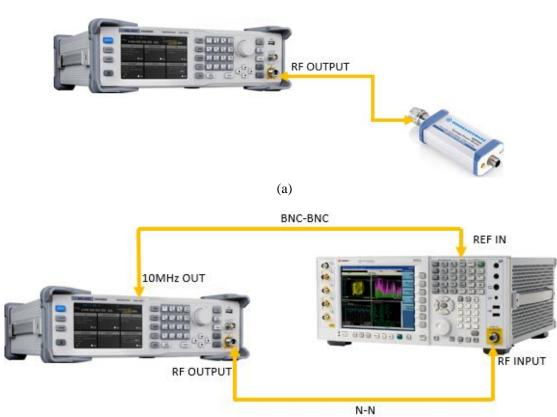
Figure 3-1 Absolute amplitude accuracy connections
